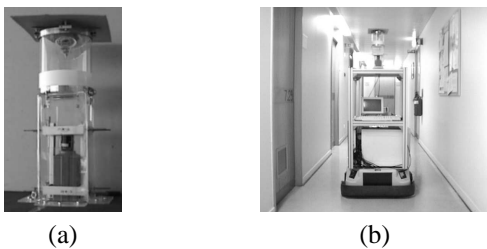
Figure 1. (a) Omni-directional camera. (b) Camera mounted on a Labmate mobile robot.
