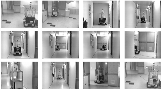
Figure 13. Experiment combining visual path following for door traversal and topological navigation for corridor following.
