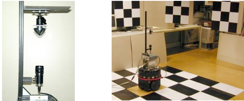
Figure 2.19: Svisca camera equipped with the combined mirror (left) and world scene with regular patterns distributed vertically and over the floor (right).
