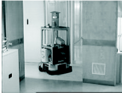
Figure 3.2: Omnidirectional vision helps in preserving features in the field of view. Even after crossing the door, some of the features of the corridor continue to be visible.
