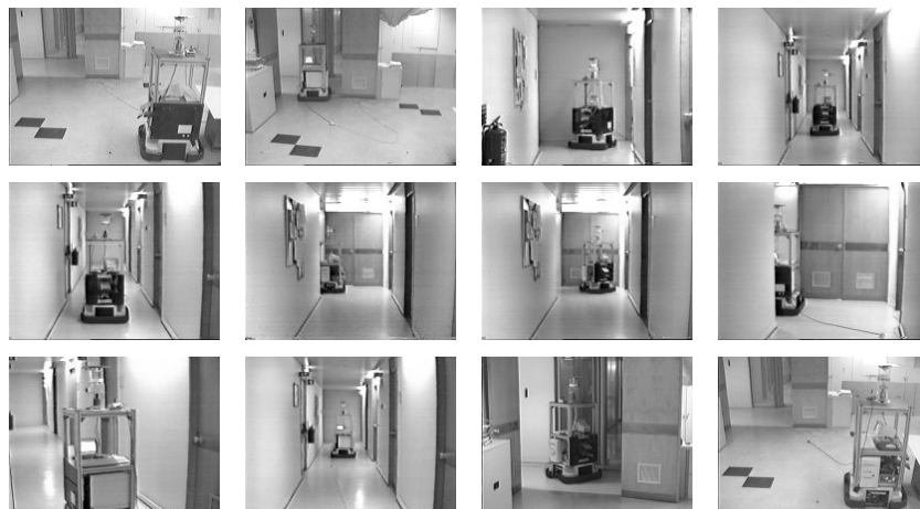
Figure 4.9: Experiment combining visual path following for door traversal and topological navigation for corridor following.
