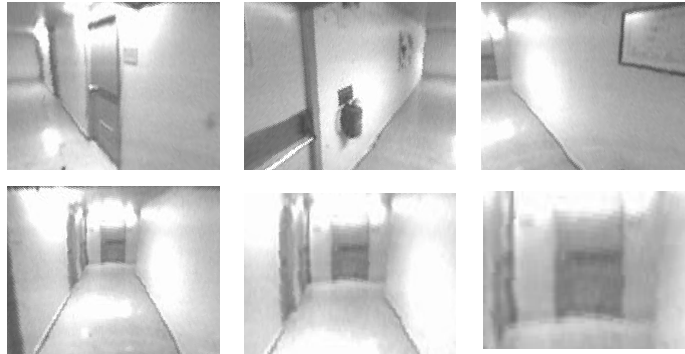
Figure 2.25: Examples of perspective images obtained from the omnidirectional image shown in Fig.2.24. On the top row the perspectives have differing directions while on the bottom row we simulated three typical focal lengths, 4.5mm, 8mm and 16mm for a 6.4x4.8mm ccd.
