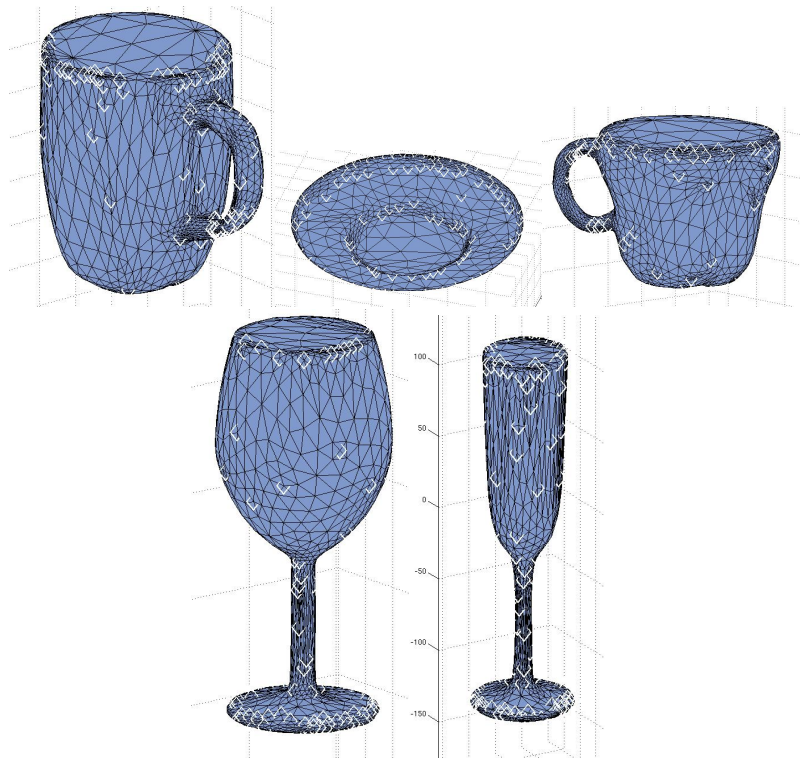
Figure 2: The white diamonds display the location of the interest points from the local maxima of the Laplacian-Beltrami operator
